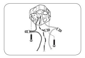
(4) Connect the three input lines (Black is L, white is N, blue and yellow is ground line) of the lamp with the output lines of the junction box.
