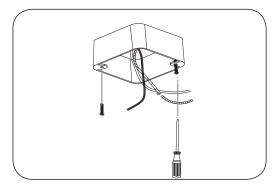
3 Drive the screws into the junction box, with 2/3 inside and 1/3 outside.
