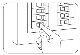
$(\ensuremath{\underline{1}})$  For safety, turn off main power prior to installation.
